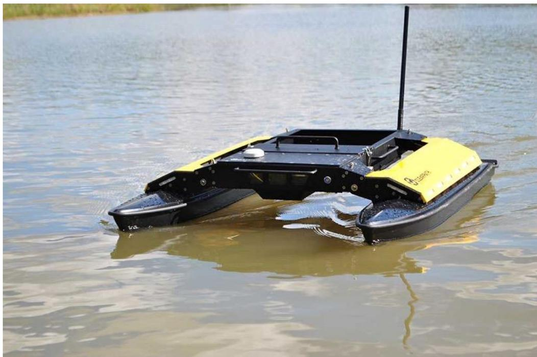
Figure 26 - Heron USV. Source: <https://clearpathrobotics.com>
