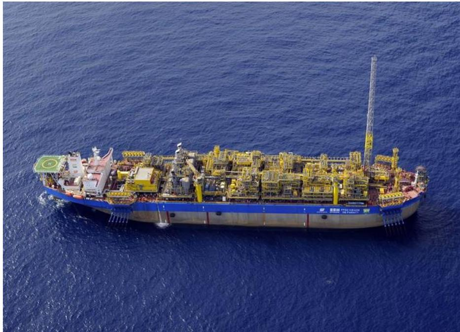
Figure 34 – FPSO unit installed on the ocean. Source: <https://petrobras.com.br/en/news/oil-and-natural-gas-output-in-february.htm>.
