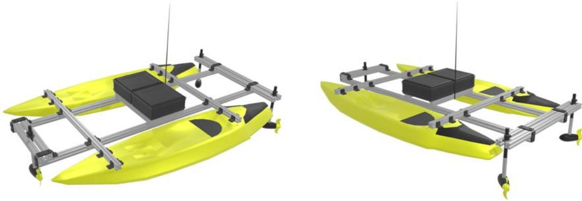
Figure 37 - 3D model of the Autonomous System on the Kayaks.
