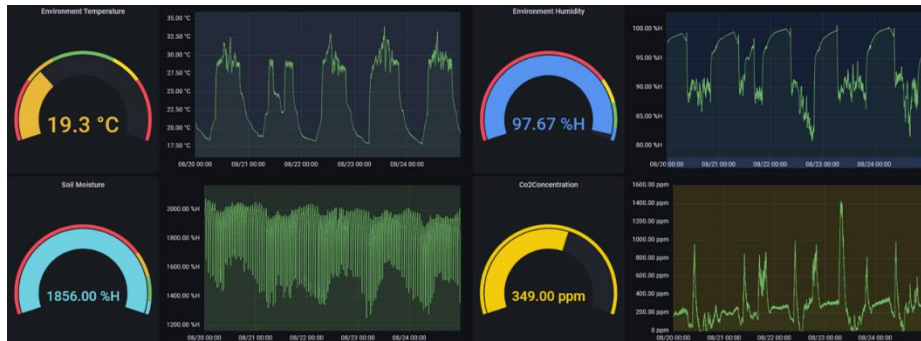
Fig. 3. Grafana dashboard showing temperature, humidity, soil moisture, and CO2
