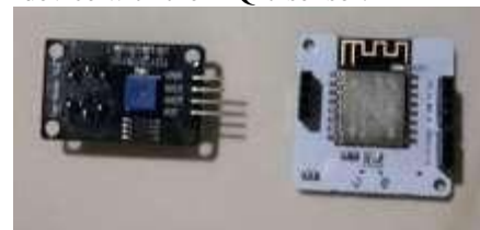
Figure 6: Bolt IOT device with MQ-7 sensor
