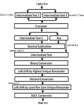
Fig. 8. Block Diagram of Decryption Process
