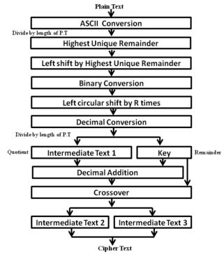
Fig. 7. Block Diagram of Encryption Process
