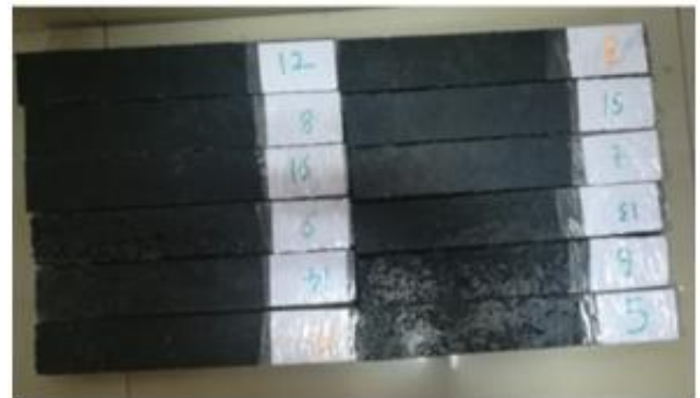
Figure 2: Specimens prepared by different combinations of epoxy and granite
