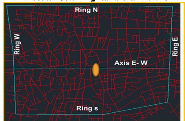
Fig 3: Axial line map showing new introduced Outer ring road and central axis
