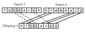
Fig. 4.Position Crossover (PX) Scheme for offspring generation from two parents.
