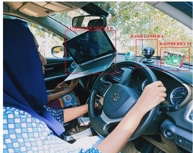
Fig. 3. Configuration of the Proposed Driver State Warning Control System on a prototype car
