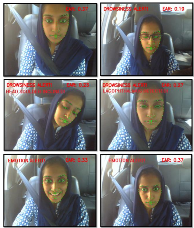
Fig. 4. (a) Screenshot of image, during which eye is open and corresponding EAR is calculated and shown on prime right.
