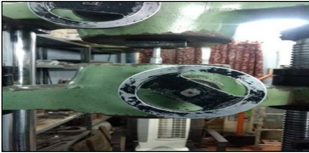
Fig 4 Specimen attached in UTM for tensile test
