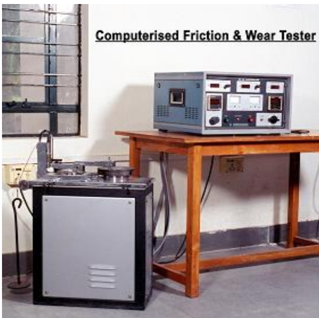
Fig 5: Computerized Pin on disc setup
