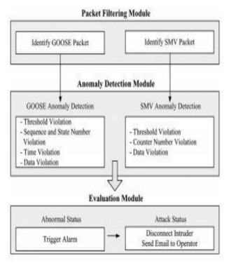
**Figure.1: Packet filtering internal Process**
