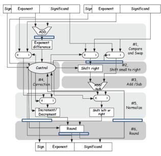
**Fig 15 : Pipelined Floating Point Addition Architecture** The proposed pipelined floating point addition architecture is shown figure 15 .The pipelined register are placed in the task to be performed . Consider two operands A and B , the XOR involves in SIGN CALCULATION : if the number is positive then its "0" else "1.
