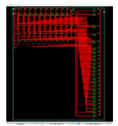
Fig 34: Technology schematic 24 bit CLA for mantissa
