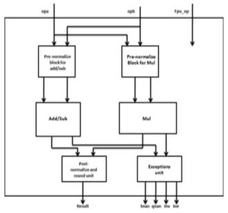
Fig 2: Architecture of proposed FPU
