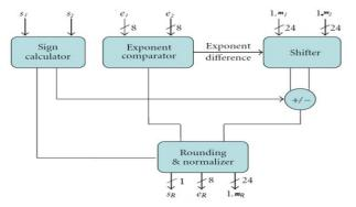
Fig 9 : Block Diagram Of Addition Unit
