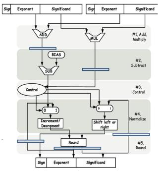
Fig 12 : Pipelined Floating Point Multiplication Architecture
