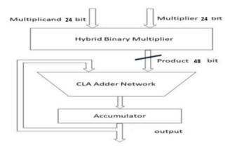
Fig 7 : 24 Bit hybrid multiplier for Mantissa
