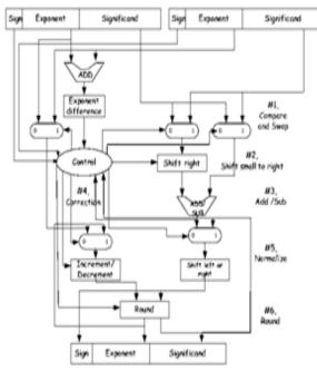
Fig 8 : Floating Point Addition Architecture
