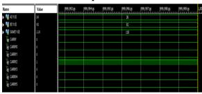
Fig 50: Simulation results of 12 bit CLA adder for exponent
