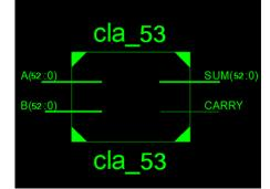
Fig 51 : RTL Design 53 bit CLA for mantissa
