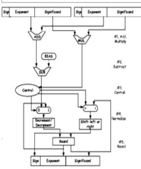
Fig 4 :Floating Point Multiplication Architecture
