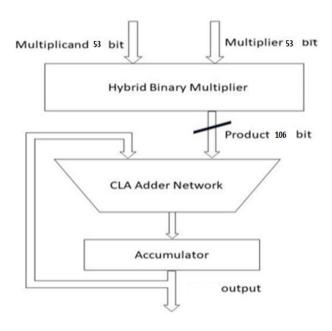
Fig 14: 53 Bit Hybrid Multiplier For Mantissa MANTISSA CALCULATION: In this design operands A and B mantissa/significand are to be multiplied.
