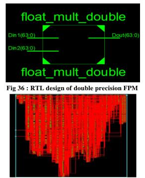
Fig 37: Technology schematic of double precision FPM
