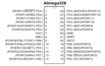
Figure1: Pin description of ATMEGA 328P Microcontroller.
