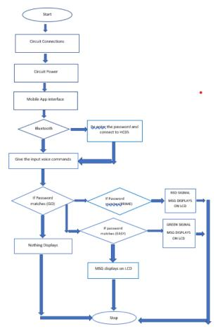
Figure 2: Showing Flow Chart of Notice Board controlled by Voice Commands
