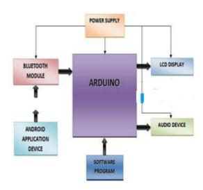
Figure 5: Block Diagram showing the notice board setup
