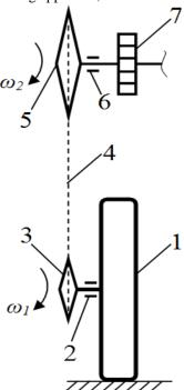
1-wheel support, 2, 6-bearing, 3-wheel sprocket; 4-flail; 5-driven sprocket; 7-disc meter
