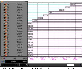
Fig 6 Waveform of ALU and memory interface
