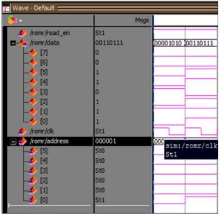
Fig 11 Waveform instruction and data memory block (ROM)
