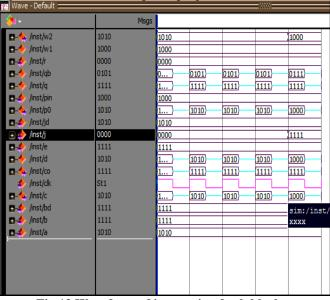
Fig 13 Waveform of instruction fetch block
