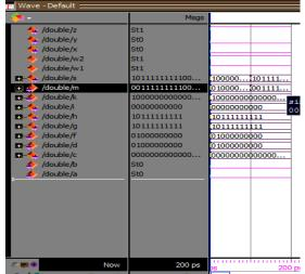
Fig 7 Waveform of floating point addition with double precision.
