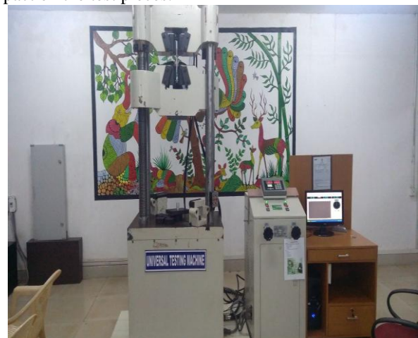
Fig. 3. Tensile test on Universal Testing Machine
