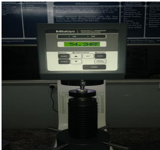
Fig. 4. Hardness test on Rockwell hardness testing machine
