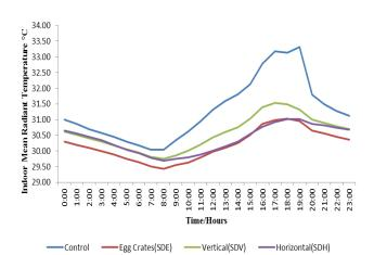
Fig. 7: Comparison of mean radiant temperature (T<sub>mrt</sub>) generated by each room on the sun-shading performance recorded in one month (May 2019).
