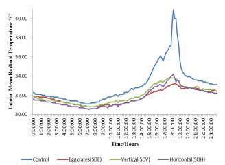
Fig. 6: Comparison of mean radiant temperature (T<sub>mrt</sub>) generated by each room on the sun-shading performance recorded on 7 May 2019.
