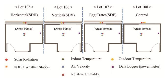
Fig. 3: Floor plan showing the position of instruments set up at the research area.
