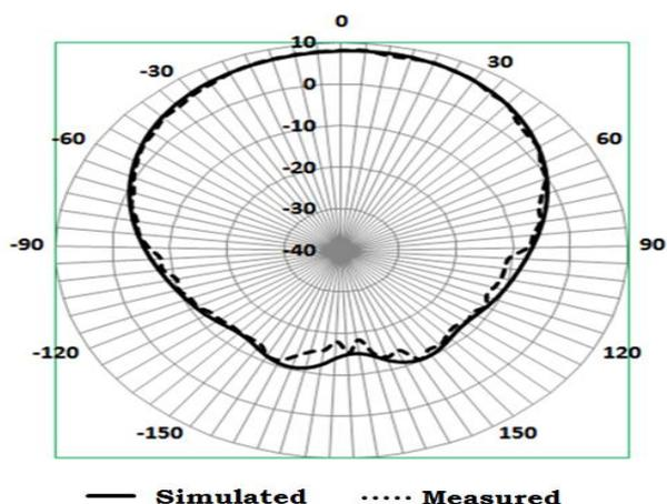
Fig. 7 Radiation patterns of RMPA in E-plane for  $\epsilon_{r2} = 2.2$ ,  $\Phi = 0$ ,  $f_r = 2.34$  GHz
