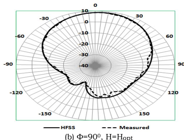
Fig 9: Measured and simulated radiation patterns (a) In E-plane for  $\epsilon_{r2} = 2.2$ ,  $h_2 = 1.6$  mm at  $H = 0$ mm (b) In H-Plane  $\epsilon_{r2} = 4.8$ ,  $h_2 = 1.6$  mm at  $H = H_{opt}$
