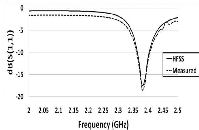
Fig 8: Return loss for RMPA with superstrate  $\epsilon_{r2} = 4.8$ ,  $h_2 = 1.60$  mm
