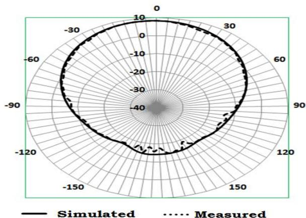
Fig. 5 Radiation patterns for RMPA in E-plane  $\epsilon_{r1} = 2.2$  without dielectric superstrate at 2.40 GHz.
