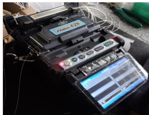
Fig-3 Splice arrangement Fujikura 62S splicer
