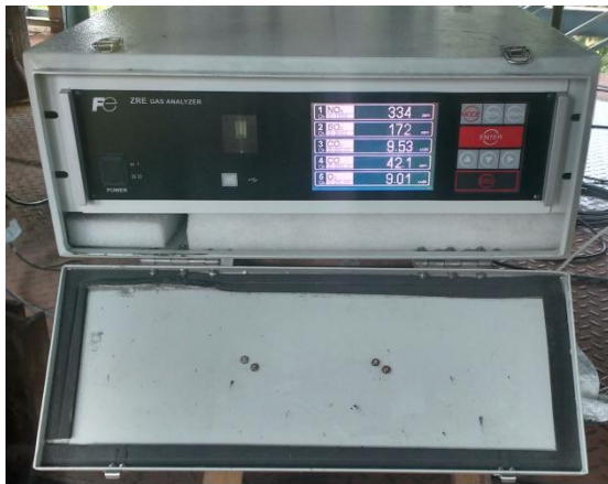
Figure 2(a) Flue Gas analyser.
