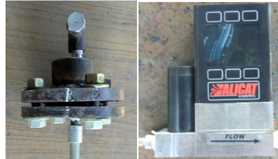
Figure 3(a) Ammonia Injection Nozzle & (b) Ammonia Mass flow Controller.
