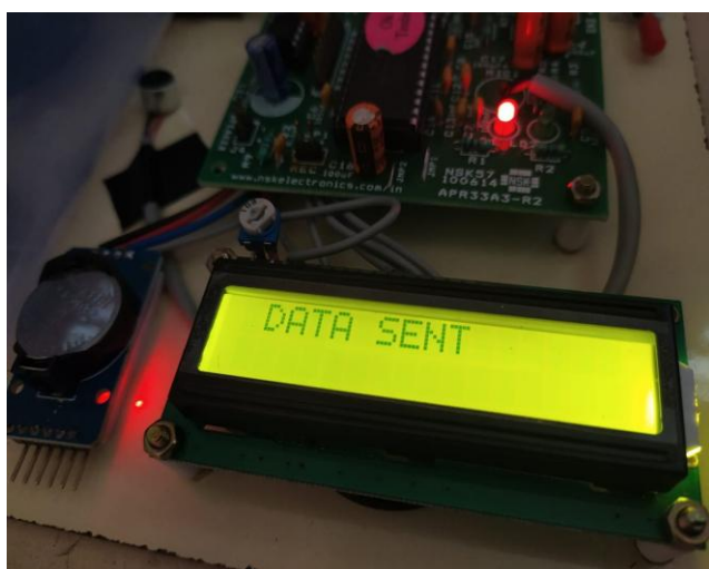
Fig 11. LCD displays the status of data sent for storage purpose
