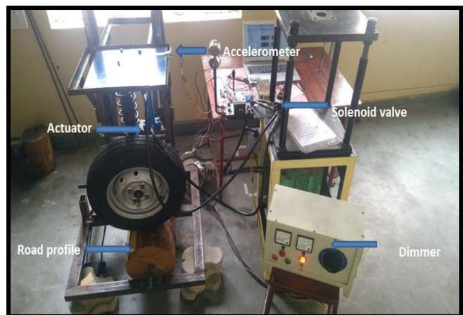
Figure 18. Experimental Setup
