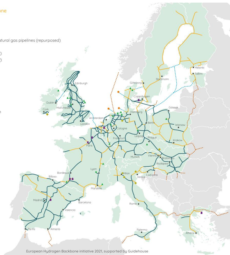
Figure 5 - Proposed European Hydrogen Backbone to provide a pan-European (21 countries) infrastructure for hydrogen in 2040 [21].
