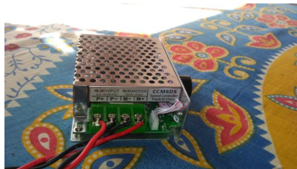
Figure 4. Connection of speed controller
