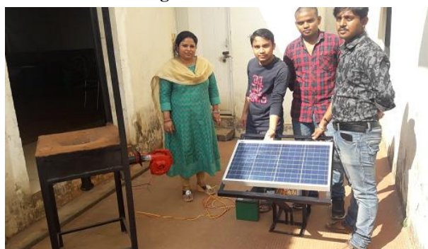
Figure 6. Full assembly of solar operated blower for forging operation
