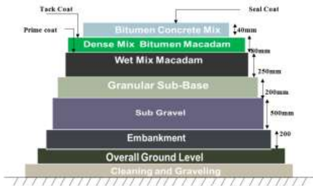
Figure 1: Different layers of flexible pavement
