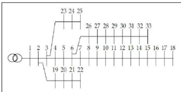
**Fig 1.7 : Single line diagram of IEEE 33 bus**
