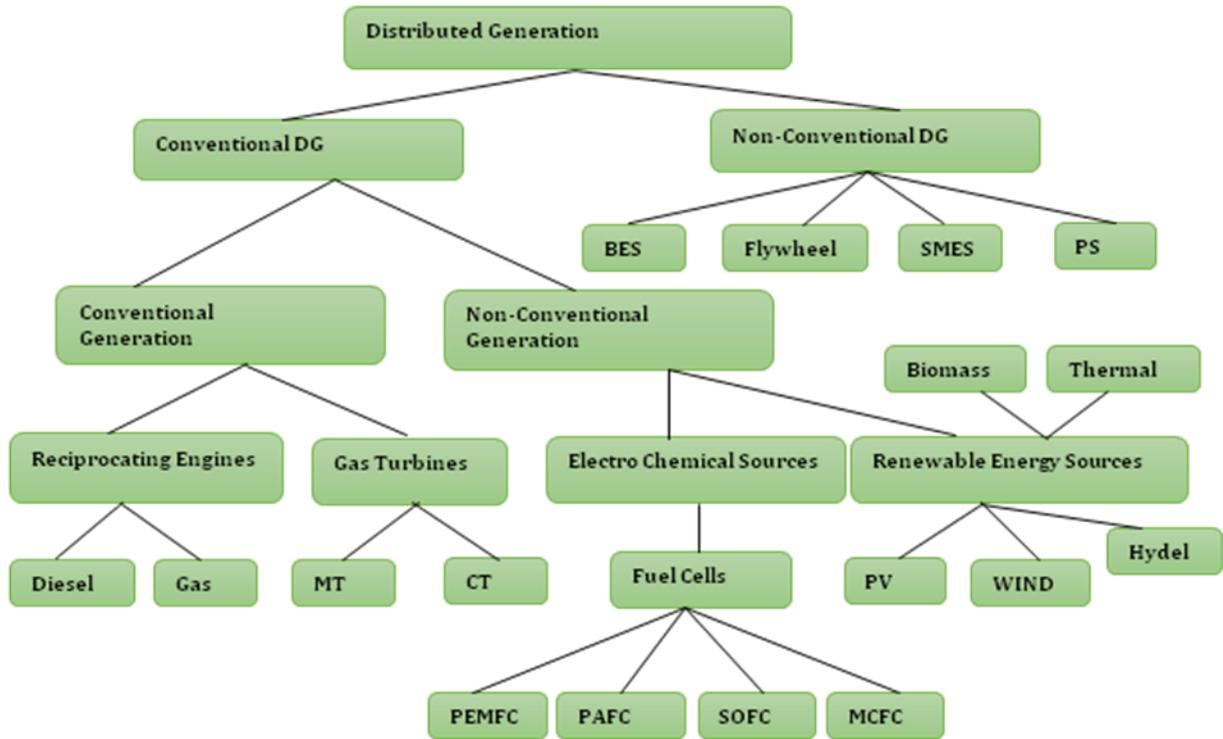
Figure 1.1: Different types of DG Technologies
