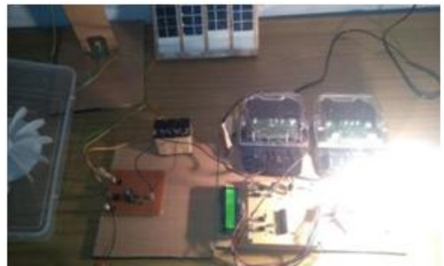
Fig. 6. LCD displaying the energy utilized for home loads (indicated as HOME) and energy given to utility grid (indicated as GOVT)
