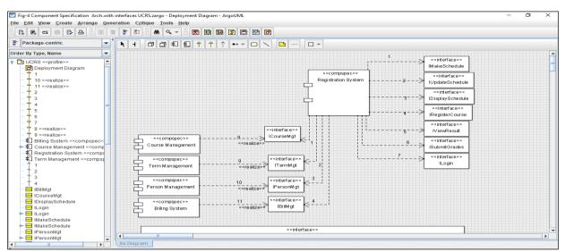
Snapshot 1. Component Diagram of UCRS Registraton System (Jawwad W.Shareef et al., 2012)
