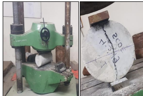
Fig. 3. Specimen before and after the failure in tension test
