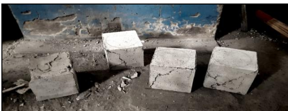
(b) Specimen after the test Fig. 1. Compression test on RPC
