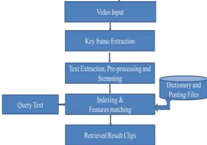
**Figure 2 Proposed Text query-based Video Retrieval Approach**
