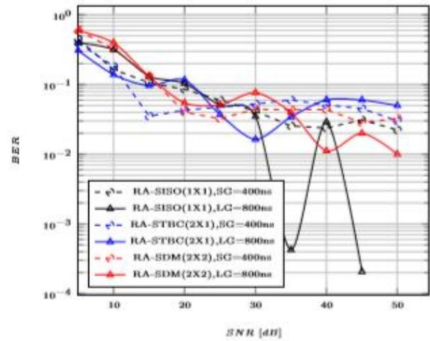
Figure 7. BER v/s SNR over TGn D channel with NLOS
