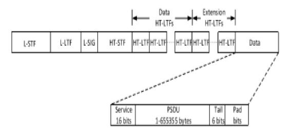
Fig 1. HT-mixed packet structure
