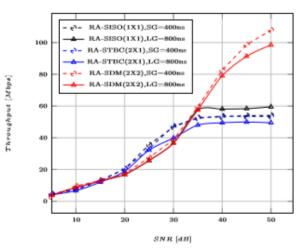
Fig 2. Throughput v/s SNR over TGn B with LOS
