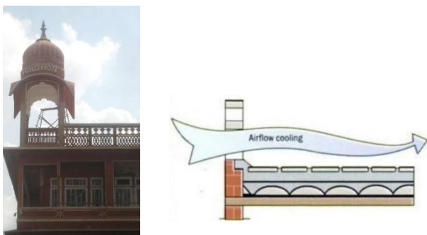
Fig. 2: Traditional elements for controlling roof temperature through solar shading and convective cooling. Source: author,[10]
