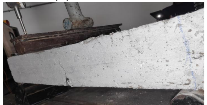
Fig.4. Testing of specimen under UTM
