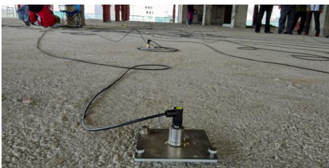
Fig. 5 Accelerometer setups at floor area A.
