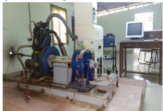
Fig-I: Computerized VCR Engine Setup with Smoke meter and Gas analyzer.
