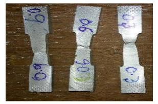
Fig. 4. Tensile specimens after test
