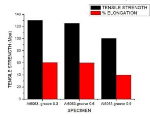
Fig. 5.Tensile strength and elongation comparison
