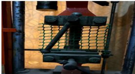
Fig. 3 Geogrid - Before Load Application
