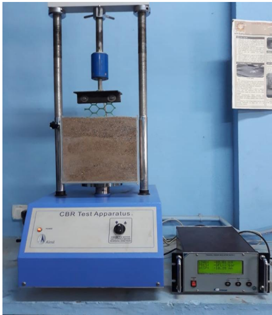
Fig. 5 Experimental setup for pullout test
