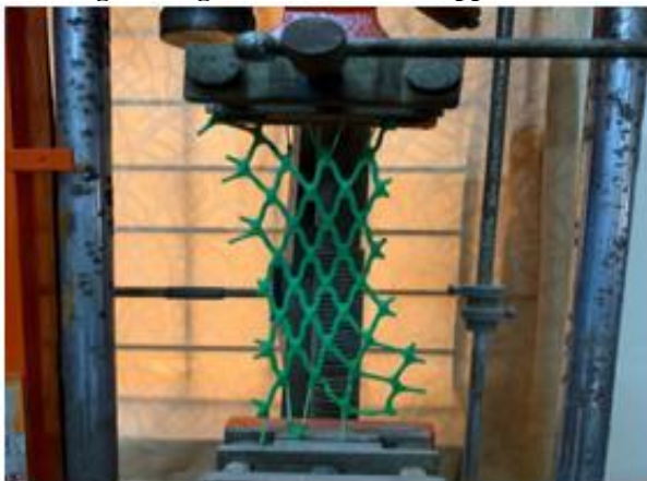
Fig. 4 Geogrid at failure
