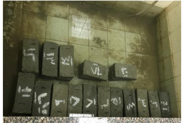
Fig. 5. Bricks immersed in water.
