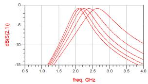
Fig. 4. Center frequency tuning response of the proposed **Q-enhanced LNA circuit.**
