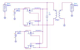
Fig. 3.Proposed Q-enhancement coupled-transformer tuning circuit.
