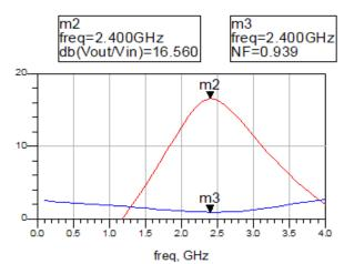
Fig. 5. Response for the proposed Q-enhanced LNA circuit Forward Gain S21 and Noise Figure at frequency 2.4 GHz.
