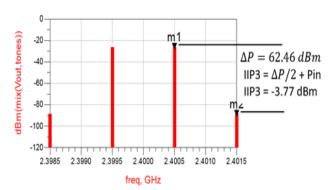
Fig. 8. Response of third-order intermodulation distortion of the proposed Q-enhanced LNA circuit at 2.4 GHz after distortion cancellation.
