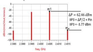
Fig. 7. Response of third-order intermodulation distortion of the proposed Q-enhanced LNA circuit at 2.4 GHz
