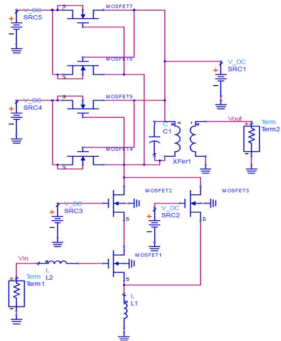
Fig. 1. Proposed fully-integrated tunable Q-enhanced LNA resonator circuit with distortion transistor compensator.
