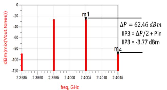
Fig. 8. Response of third-order intermodulation distortion of the proposed Q-enhanced LNA circuit at 2.4 GHz after distortion cancellation.
