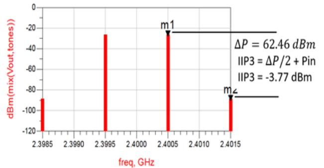
Fig. 7. Response of third-order intermodulation distortion of the proposed Q-enhanced LNA circuit at 2.4 GHz
