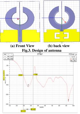
Fig .4 The return loss of the antenna
