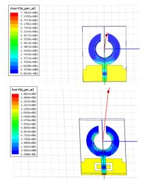
Fig.2. Current distribution of the constructed antenna
