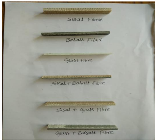
Fig. 4 Shows Flexural specimen before fracture
