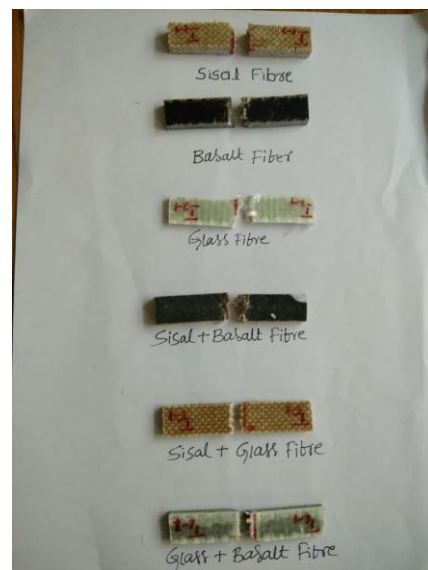
Fig.8 Shows Impact specimen after fracture
