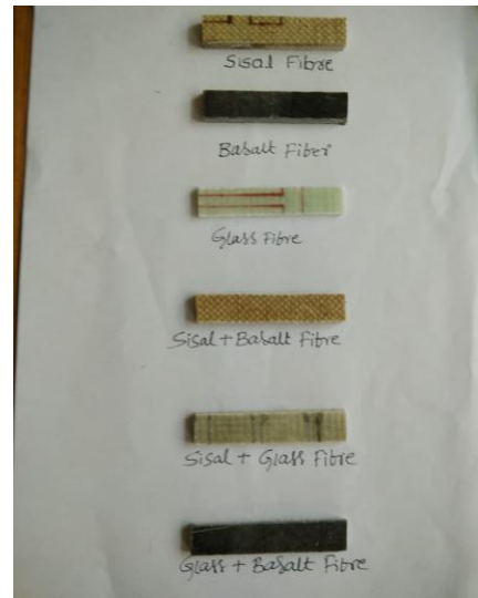
Fig.7 Shows Impact specimen before fracture
