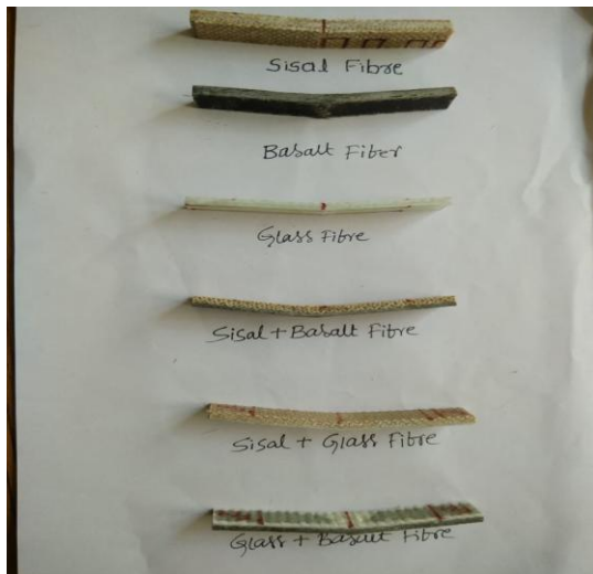
Fig.5 Shows Flexural specimen after fracture
