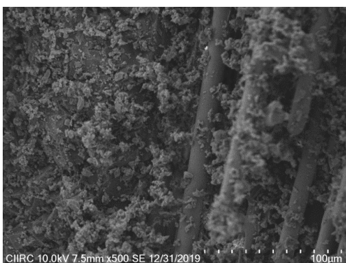
Fig. 13 shows SEM images of Sisal+Glass fiber
