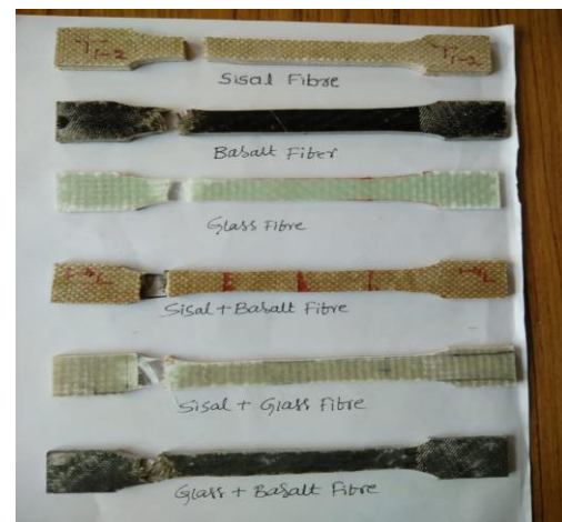
Fig.2 Shows Tensile specimen after fracture
