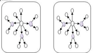
Figure 2: MPR based packet flooding in OLSR
