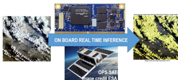
Figure 1: 22nd March 2021: the first image inferred on-board by an Artificial Neural Network running on OPS-SAT System On Chip (Cyclone V)
