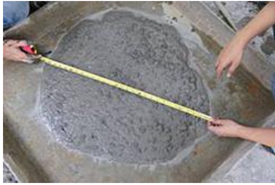
Fig 1: Slump flow of SCC
