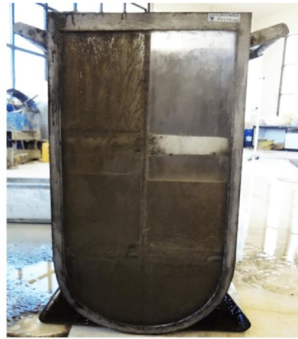
Fig 4: U-Box test of SCC
