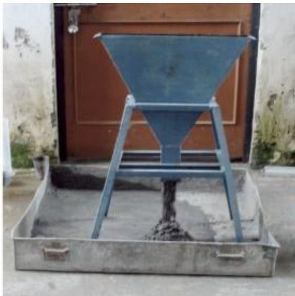
Fig 2: V-funnel test on SCC
