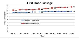
Fig. 7.3 Chart showing the reduction in indoor temperature in room no. 106
