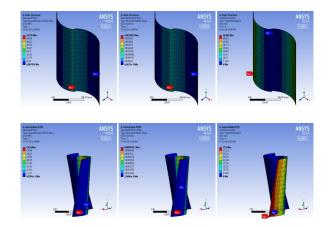
Fig.5 : Stress, Strain and Total Deformation for R350 mm and Twisted with R250 mm in 1000N loads for Steel
