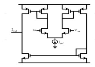
Fig. 3. CMOS circuit design of Mapping circuit
