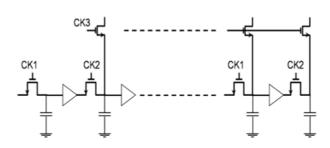
Fig. 2. CMOS circuit design of sample and hold circuit
