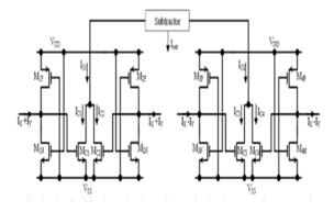
Fig. 6. CMOS circuit design of synapse using multiplier
