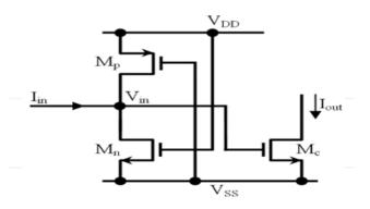
Fig. 5. CMOS circuit design of quadratic cell
