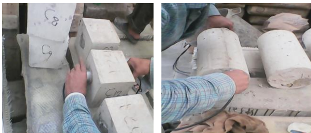
a) Cube C_p Measurement b) Cylinder C_p Measurement Fig.6: Measuring Ultrasonic Wave Velocity through Cubes and Cylinders
