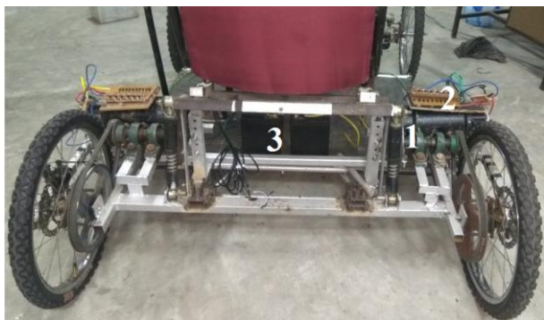
Fig. 10. Back-panel of NEV (1-Motor, 2-Freewheeling, 3-Battery)
